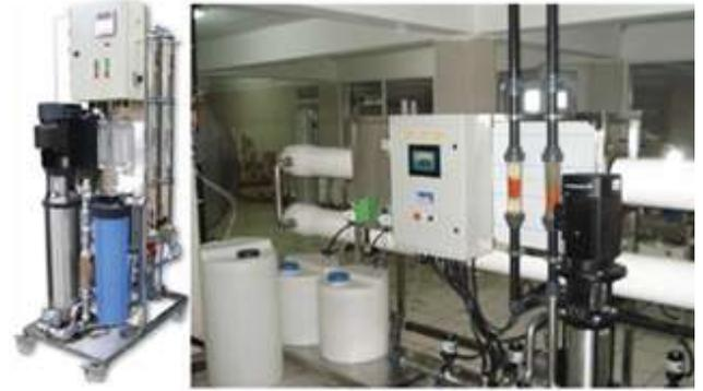
16 PVC pipes. Unit is equipped with stainless steel manometers showing pressure in water inlet, water outlet and other pressure values in unit. Housing of system can operate with 3 -10 PH water. Low and high pressure safety system combined with a conductivity alarm are present.
